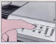
If you accidentally go past the required track, hold down the SELECT button until the TRACK Display LED runs right through and returns to track 1, then run forward to the track required.
