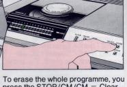
To erase the whole programme, you press the STOP/CM (CM = Clear Memory) button. All the PROGR Display LEDs light and the TRACK Display LED goes out.
