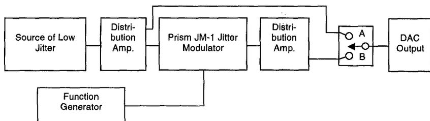
Figure 15: *Experimental Setup for Up-Down Threshold Test*
