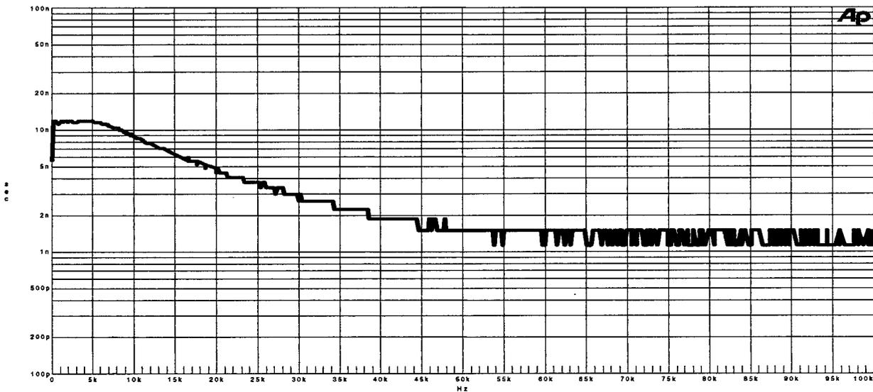
Figure 10: *Jitter Attenuation for Digital Interface Receiver with 10 ns rms Jitter vs. frequency*
