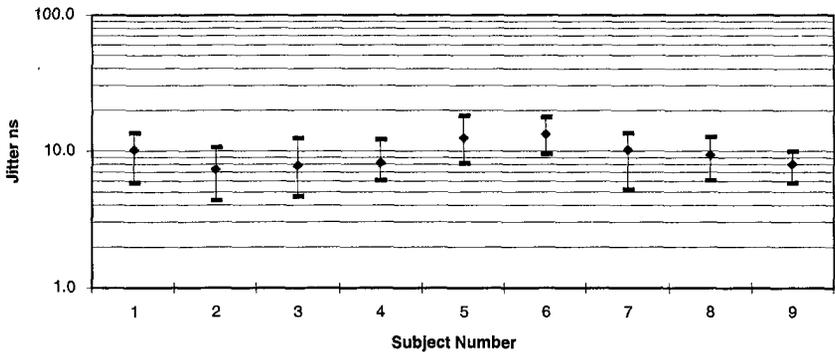
Figure 19: *Threshold of Audibility of Distortion for 20 kHz Sine Wave*
