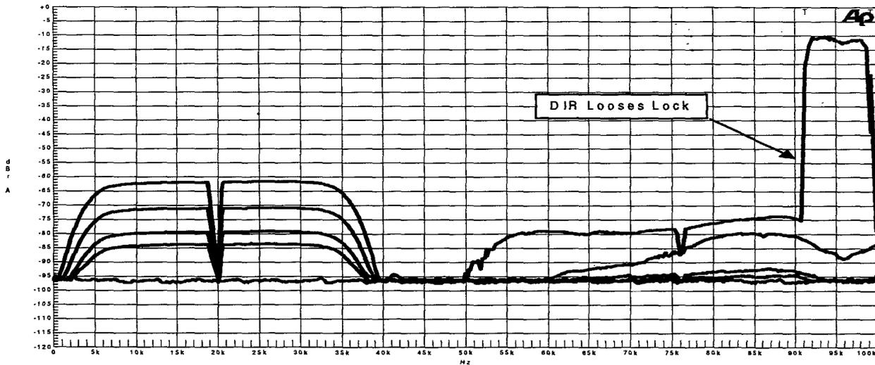
Figure 13: *Jitter Susceptibility of DAC C for no jitter, 1.6, 3, 10, and 30 ns rms jitter vs. frequency*
