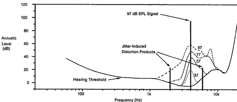
Figure 16: Masking by 4 kHz Sine Wave
