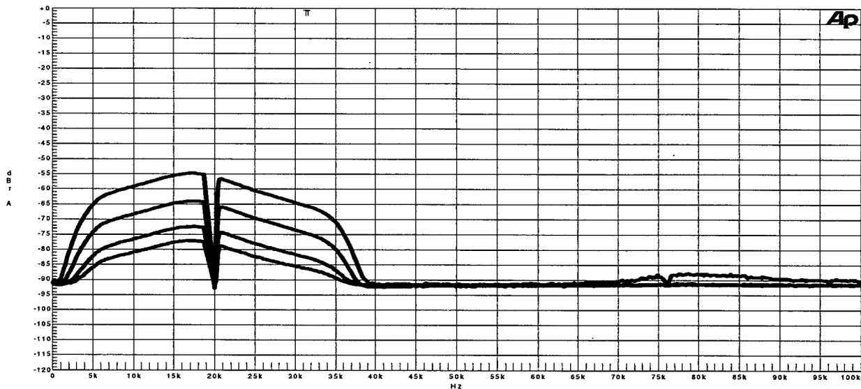
Figure 11: *Jitter Susceptibility of DAC A for 1.6, 3, 10, and 30 ns rms jitter vs. frequency*
