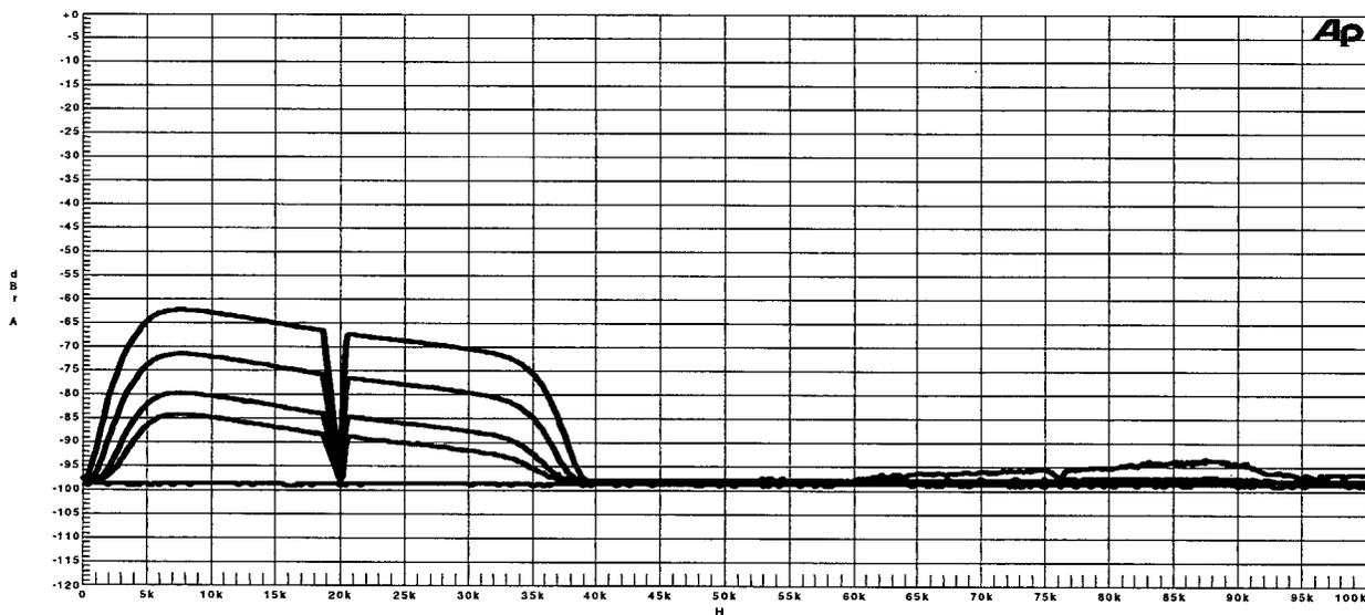
Figure 12: *Jitter Susceptibility of DAC B for no jitter, 1.6, 3, 10, and 30 ns rms jitter vs. frequency*
