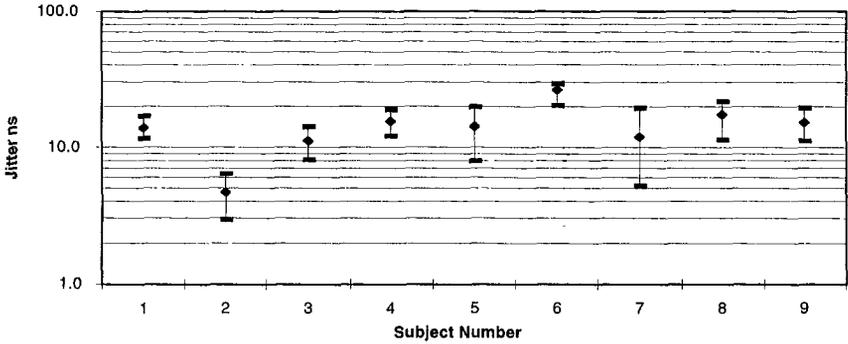
Figure 18: *Threshold of Audibility of Distortion for 8 kHz Sine Wave*
