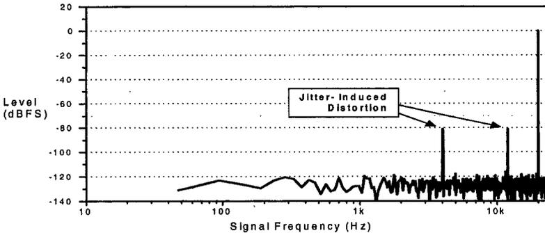
Figure 1: *Simulation of Effect of Jitter on DAC; 20 kHz at FS, 1 ns rms 16 kHz jitter*
