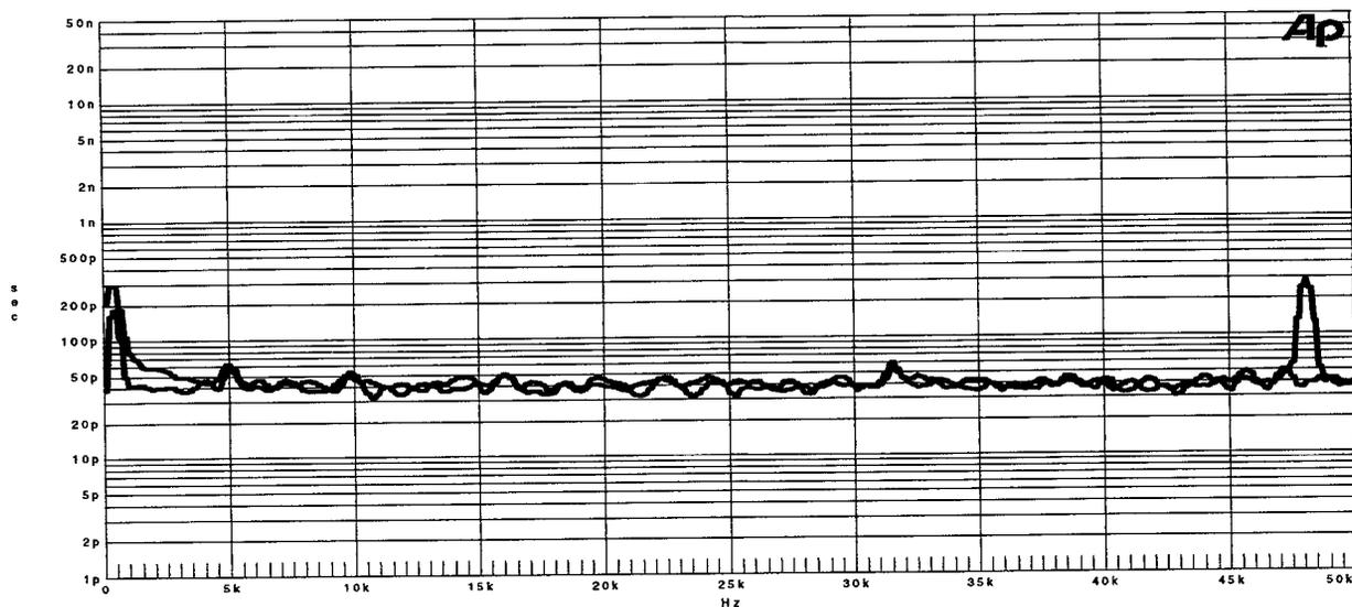
Figure 9: *Jitter in IEC 60958 Bitstream Caused by Bursts of Non-Linearly Coded Audio*
