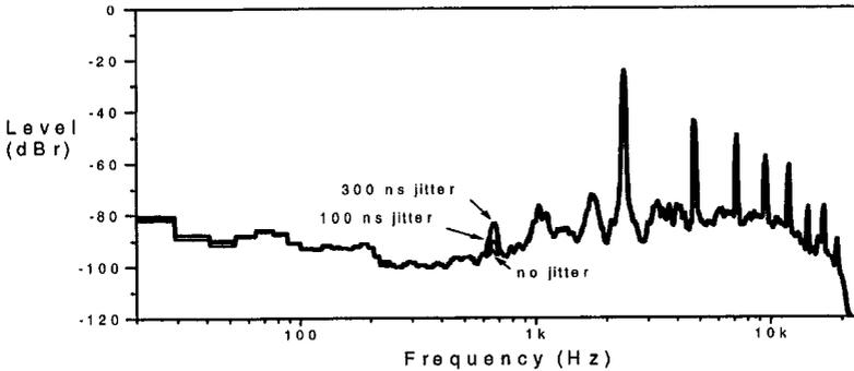
Figure 17: Audible Distortion of Piccolo Playing D4 by Addition of Sine Wave Jitter
