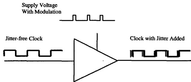
Figure 3: *Jitter Added by Supply Modulation of Gate*
