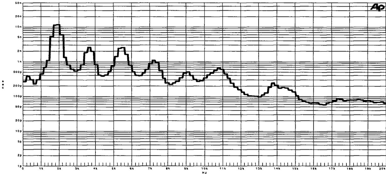
Figure 5: *Jitter Spectrum of Poor HDTV Receiver*
