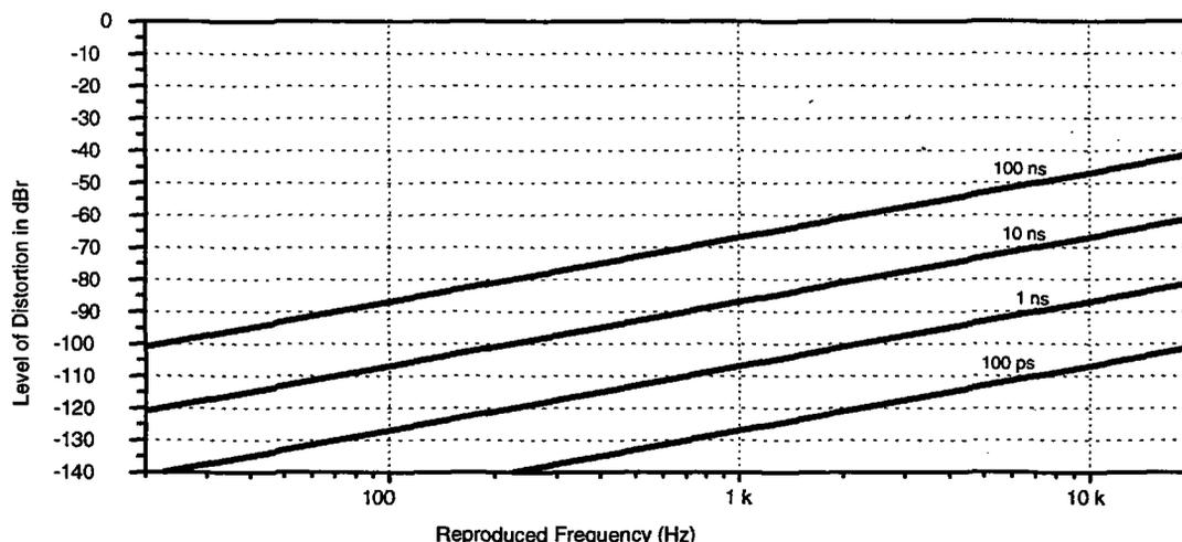
Figure 2: *Simulation of Effect of Jitter on DAC*
