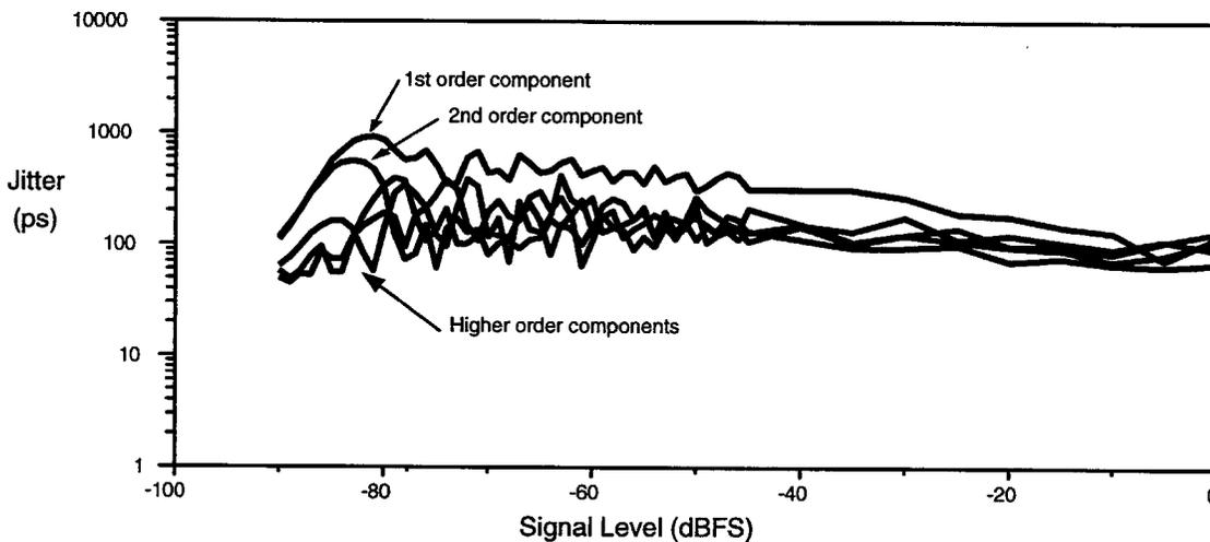
Figure 8: *Line Induced Jitter from 30 m Cable*
