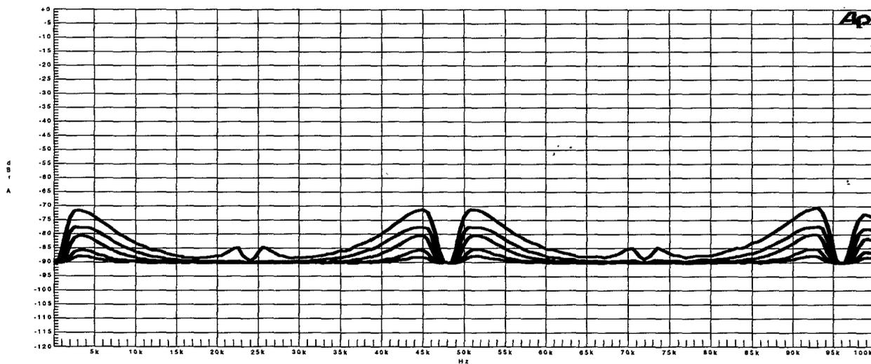
Figure 14: *Jitter Susceptibility of DAC D for 1.6, 3, 10, and 30 ns rms jitter vs. frequency*
