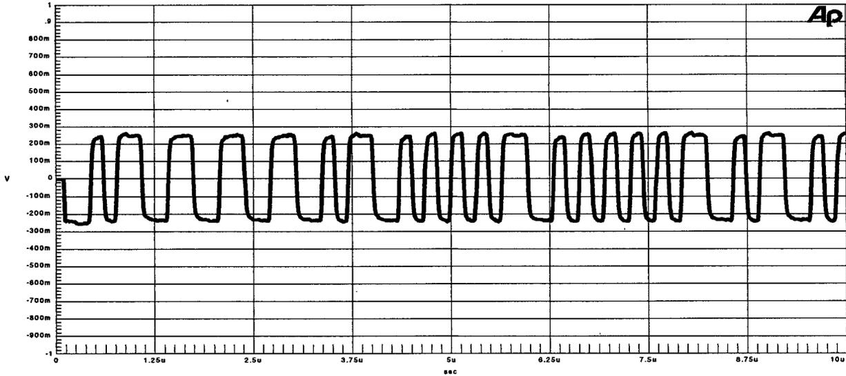
Figure 6: *Waveform from 30 m Cable Conveying IEC60958 Bitstream*
