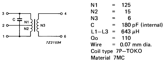
Fig. 9 IF bandpass filter (L2). TOKO sample no. 7MCS2197.
